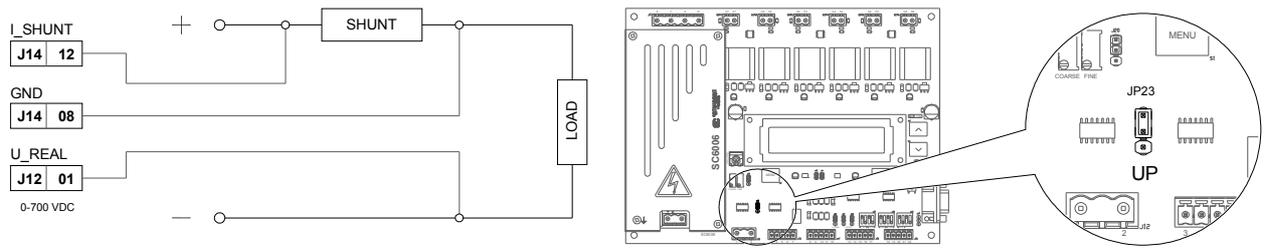
figure 33: Example of connection for shunt on positive terminal.
