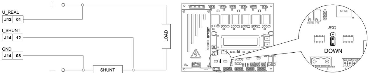
figure 34: Example of connection for shunt on negative terminal.
