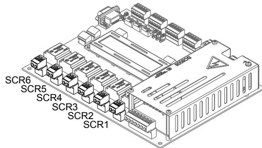
The connectors type is an MSTBVA series (or equivalent) from Phoenix Contact (ref. 1755736). The board is also provided with the matching plug connectors (ref. 1757019).
