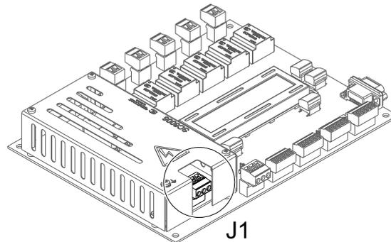
figure 13: Detail of mains supply input connector.
