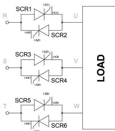
figure 26: W3C circuit connection example.
