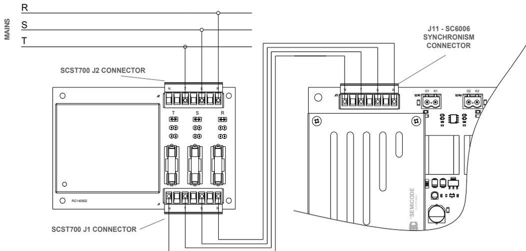
figure 39: Interfacing SC6006 with mains voltage from 200 to 700 V<sub>AC</sub>.
