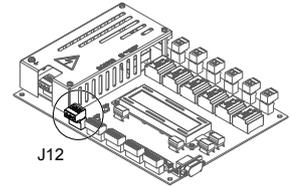
The connector type is an MSTBVA series (or equivalent) from Phoenix Contact (ref. MSTBVA2,5/3-G-5,08). The board is also provided with the matching plug connector (ref. MSTB2,5/3-ST-5,08).
