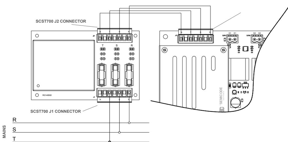
figure 40: Interfacing SC6006 with mains voltage from 65 to 200 V<sub>AC</sub>.
