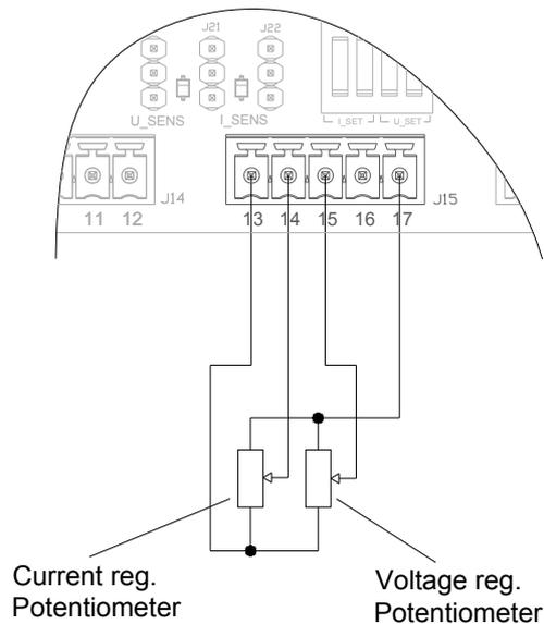
figure 17: Connection diagram example for J15.
