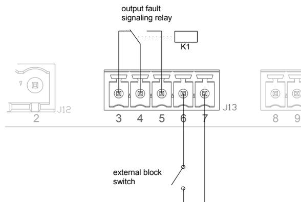
figure 15: Connection example diagram for J13.
