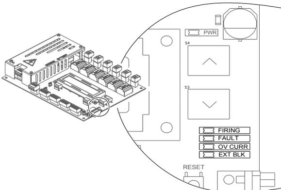
There are a total of 5 LEDs in the PCB that shows the state of the system. If it is firing, in fault mode or there is an overcurrent or blocking event:
