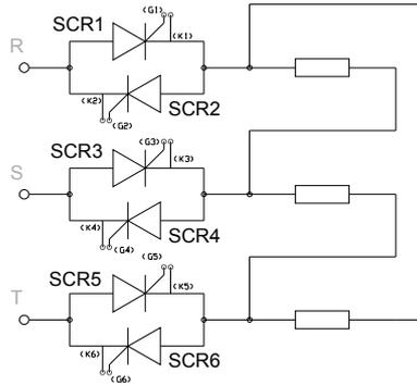
figure 29: Load in delta circuit.
