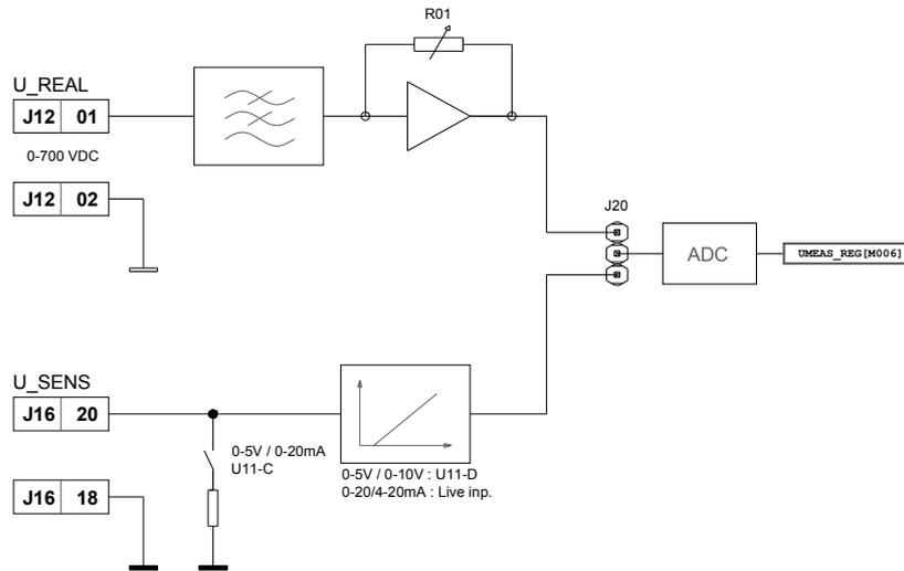
figure 8: Voltage feedback signal processing diagram.
