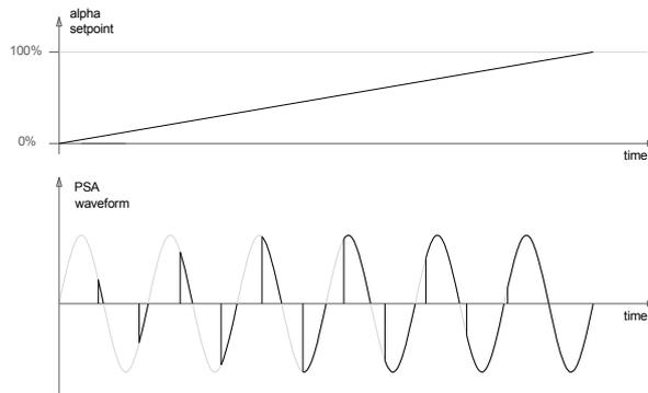
figure 1: PSA waveform example versus alpha setpoint.
