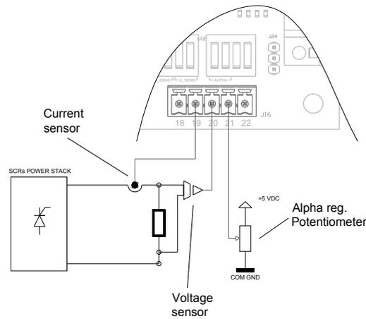
figure 18: Connection diagram example for J16.
