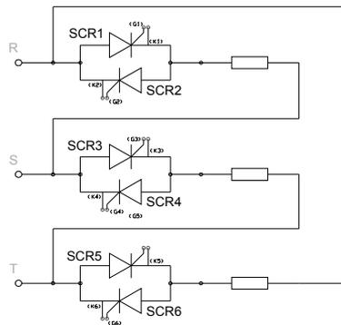
figure 30: Load in open delta circuit.
