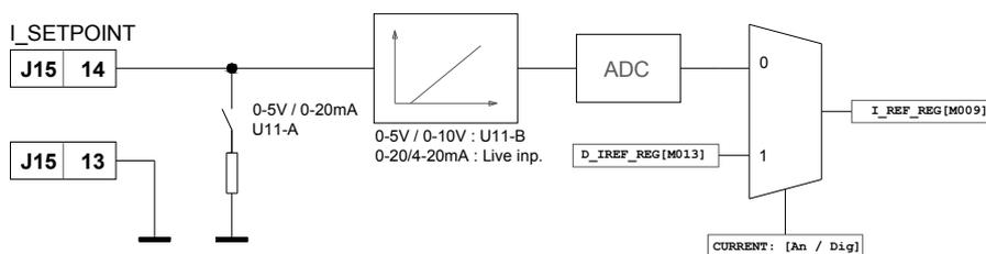
figure 6: Current setpoint signal processing diagram.
