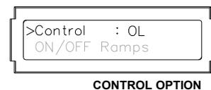
By pressing [OK] button system changes between “OL” (open loop), “I” (current regulation), “V” (voltage regulation) or “IV” (both current and voltage regulation).
