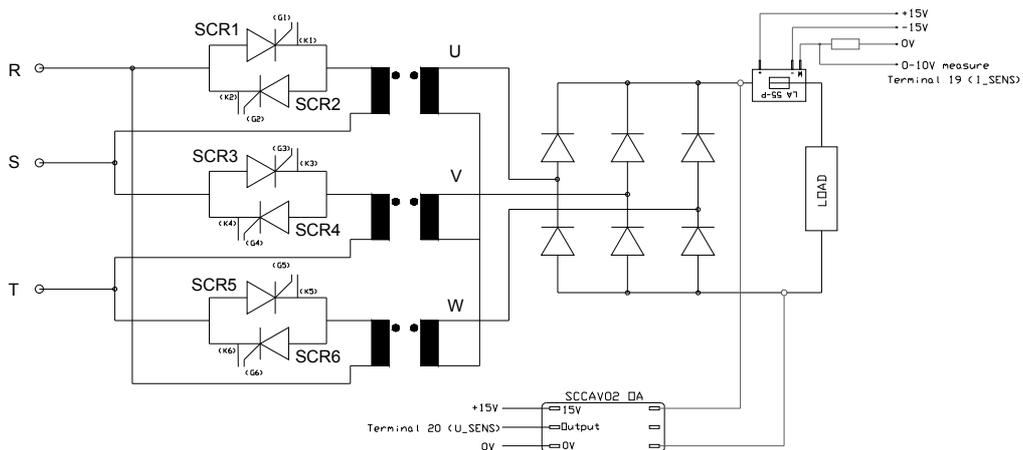
figure 35: AC/DC converter example with current and voltage feedback from transformer in primary side.
