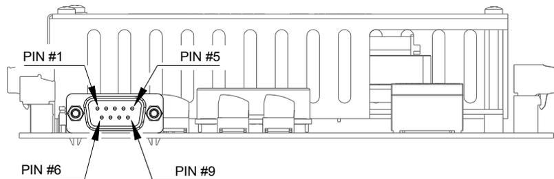
figure 25: J32 Connector (male D-SUB9) pinning detail. SC6006 lateral view.
