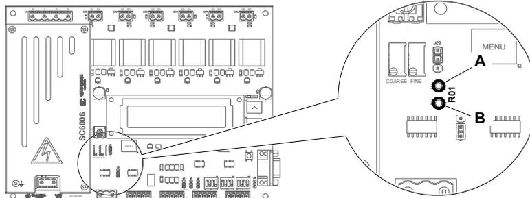
figure 24: Detail of test points for R01.
