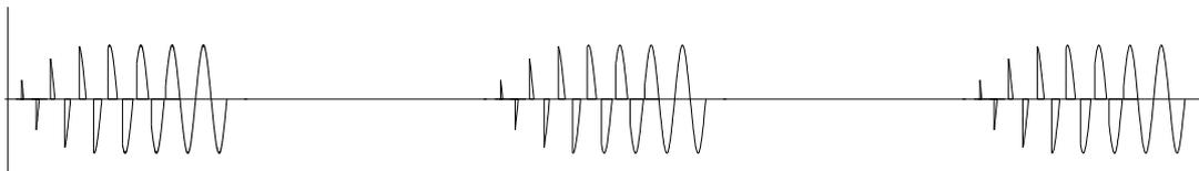
figure 10: Pulse train example with a soft init on FWS mode.
