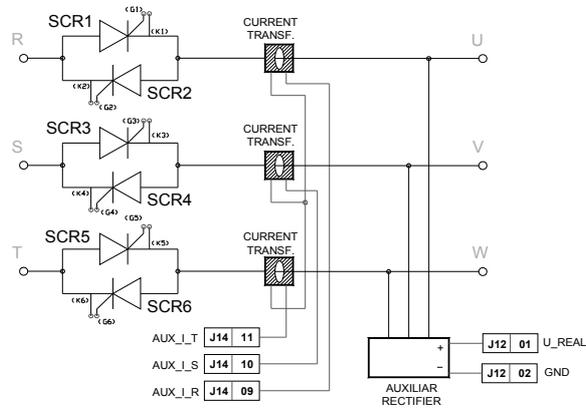
figure 27: Feedback connection W3C example.
