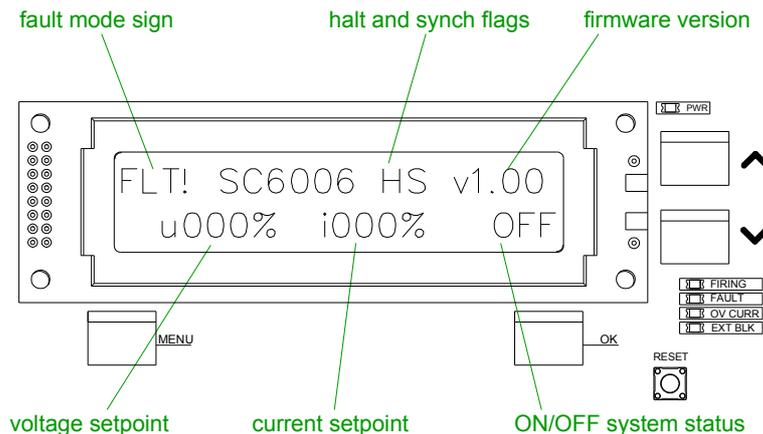
figure 21: Detail of main menu in LCD display.
