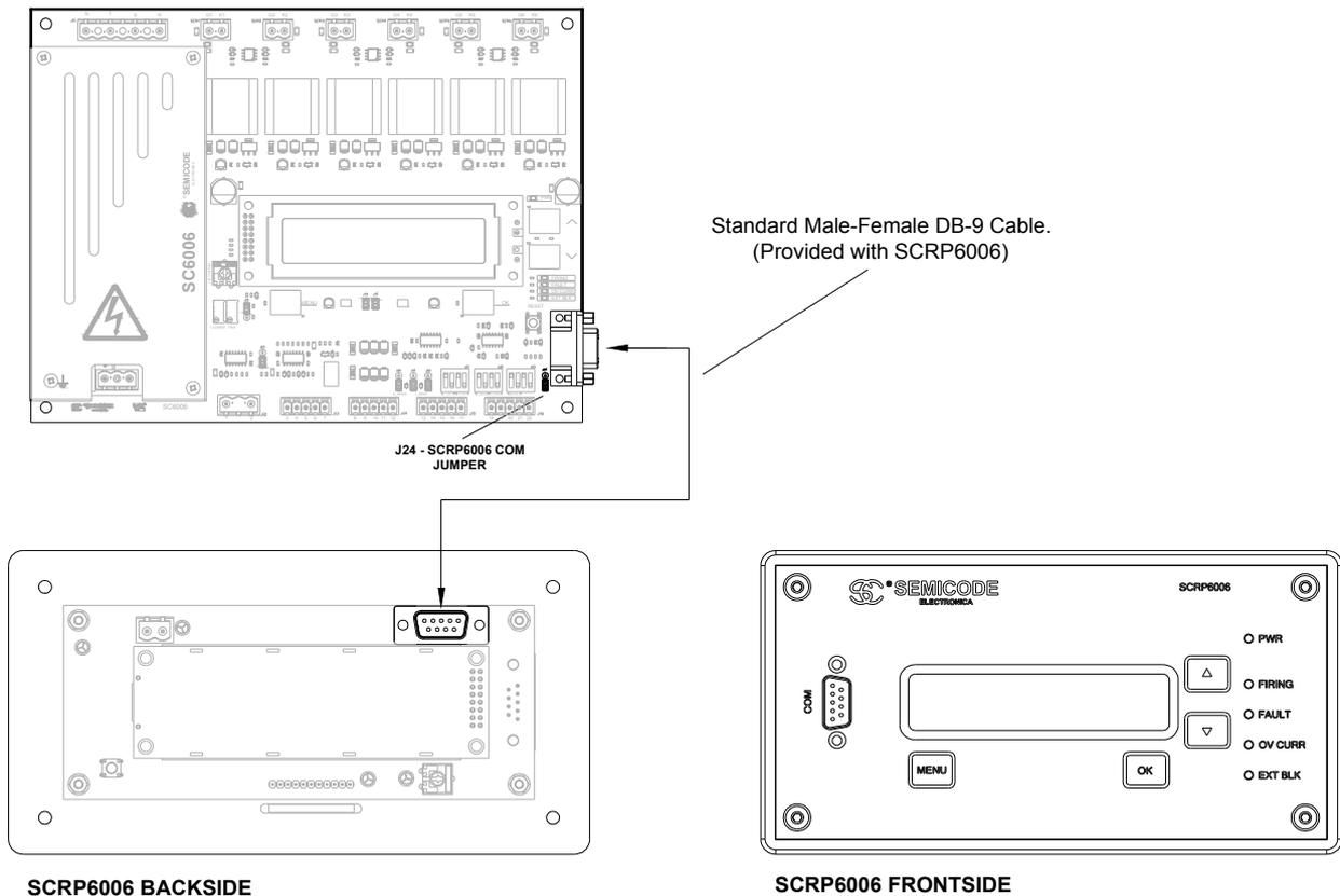
figure 37: Example of connection between SC6006 and SCRP6006.
