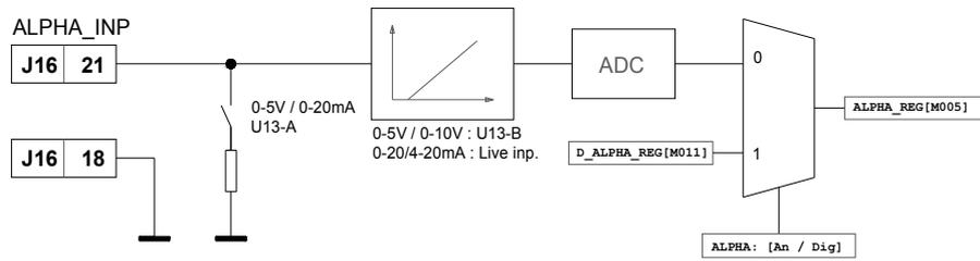
figure 4: alpha setpoint signal processing diagram.
