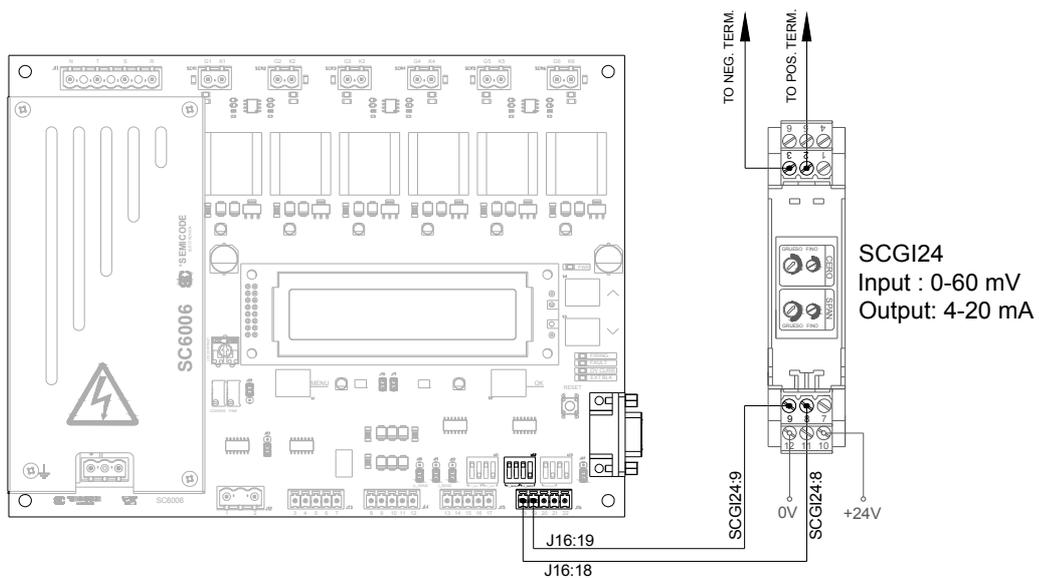
figure 38: Interfacing 60 mV shunt application with SCGI24 and 4-20 mA current loop signal.
