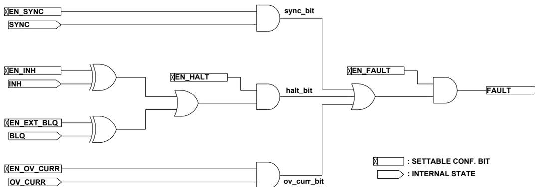
figure 11: Logic diagram for fault signal.
