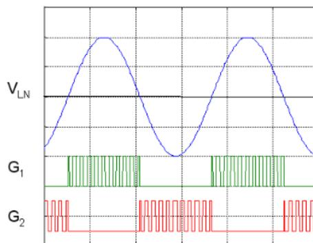
figure 3: Example of picket fence gate driving.
