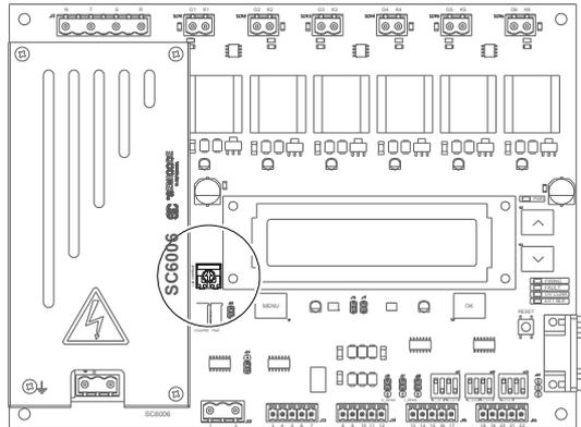
figure 22: P5 LCD contrast adjusting potentiometer
