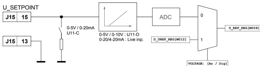
figure 5: Voltage setpoint signal processing diagram.
