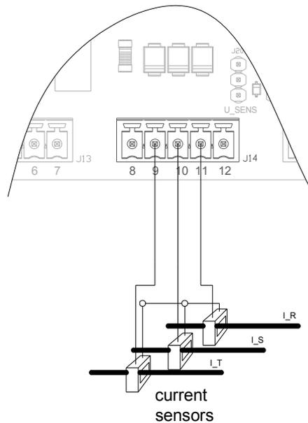
figure 16: Connection diagram example for J14.
