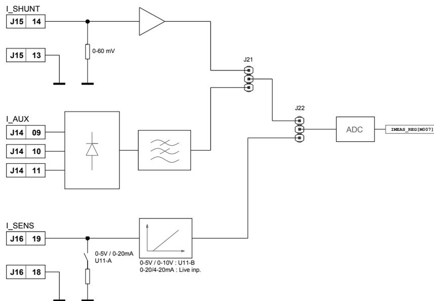
figure 7: Current feedback signal processing diagram.
