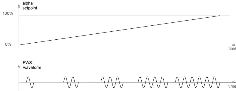
figure 2: FWS waveform example versus alpha setpoint.
