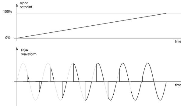
figure 9: PSA soft power on waveform example.
