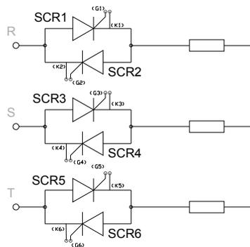
figure 28: Load in wye circuit.
