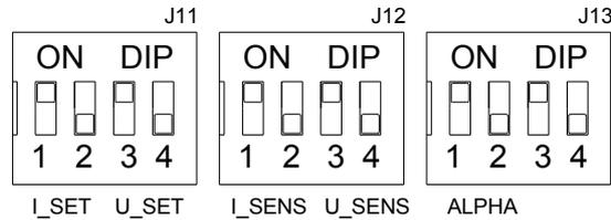
figure 23: Detail of the default configuration of DIP switches.
